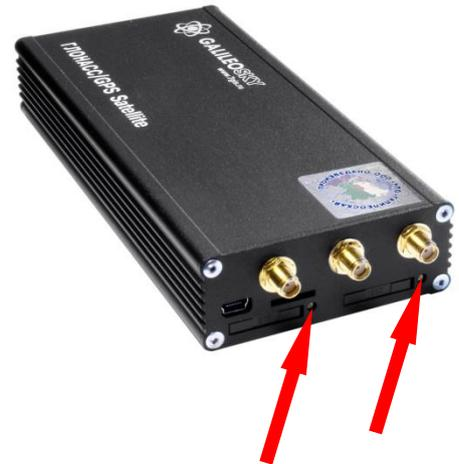
The second SIM-card should be inserted in a similar way.
