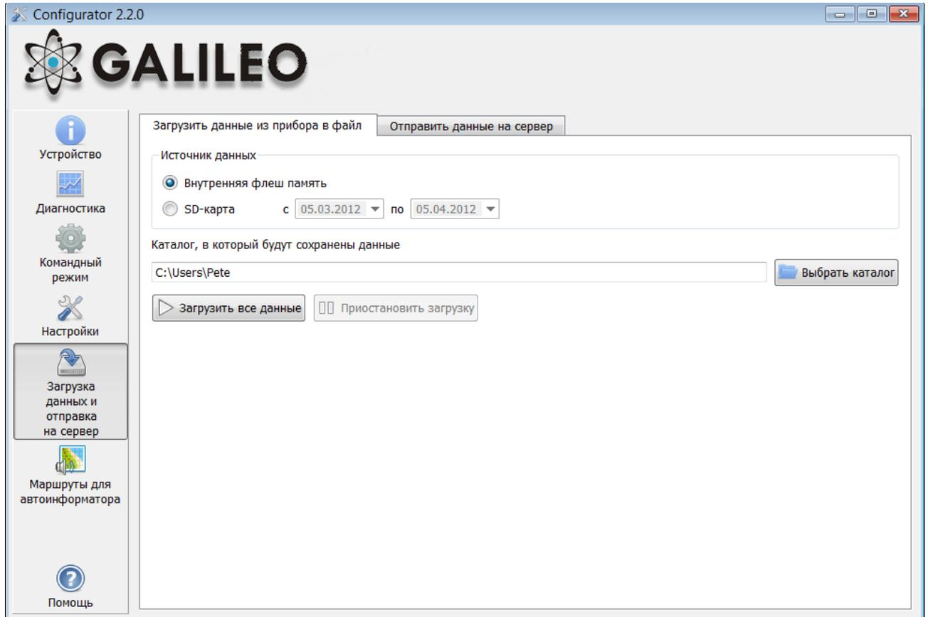
The Data transfer from the internal memory can be stopped and resumed; the data transfer from the SD card can be stopped only if you disconnect the USB cable.
