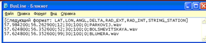
Latitude and longitude values are entered through the point "." (For example: 57.9842) where the value after point – is degree fractions. To transfer minutes into degree fractions (Xdegr.Ymin.) use the following expression  $Xdegr. = Ymin./60$ . For example: 57 degr. 55.4513min = 57.924188 degr.
