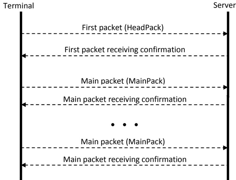
After establishing device-server connection the device sends head pack and then main packs with the data. Each pack needs conformation from the server; if confirmation is not received the terminal sends the pack once again.
