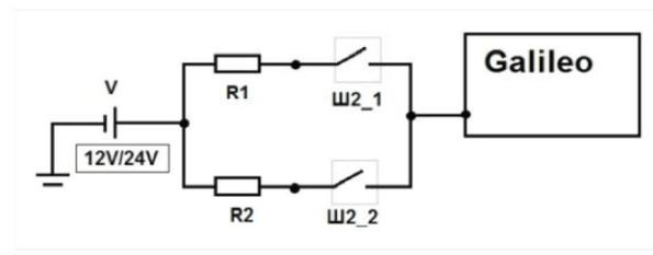
V – Power supply (battery/ vehicle power supply);
