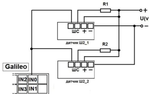
Connection order of 2 Ш2 sensors through resistors to one of DAI of the terminal.
