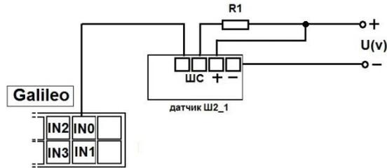
To connect 2 Ш2 sensors to one of DAI use divisor on two resistors. Calculation principle is realized on voltage level change at sensors triggering.
