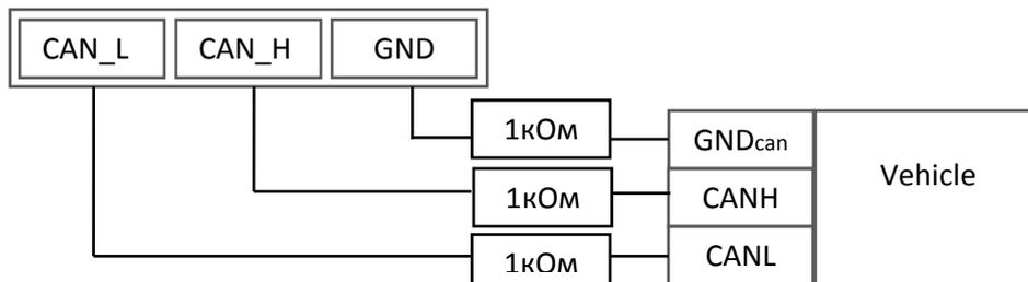
Use the first variant of connection to plug the device into the diagnostic outlet.
