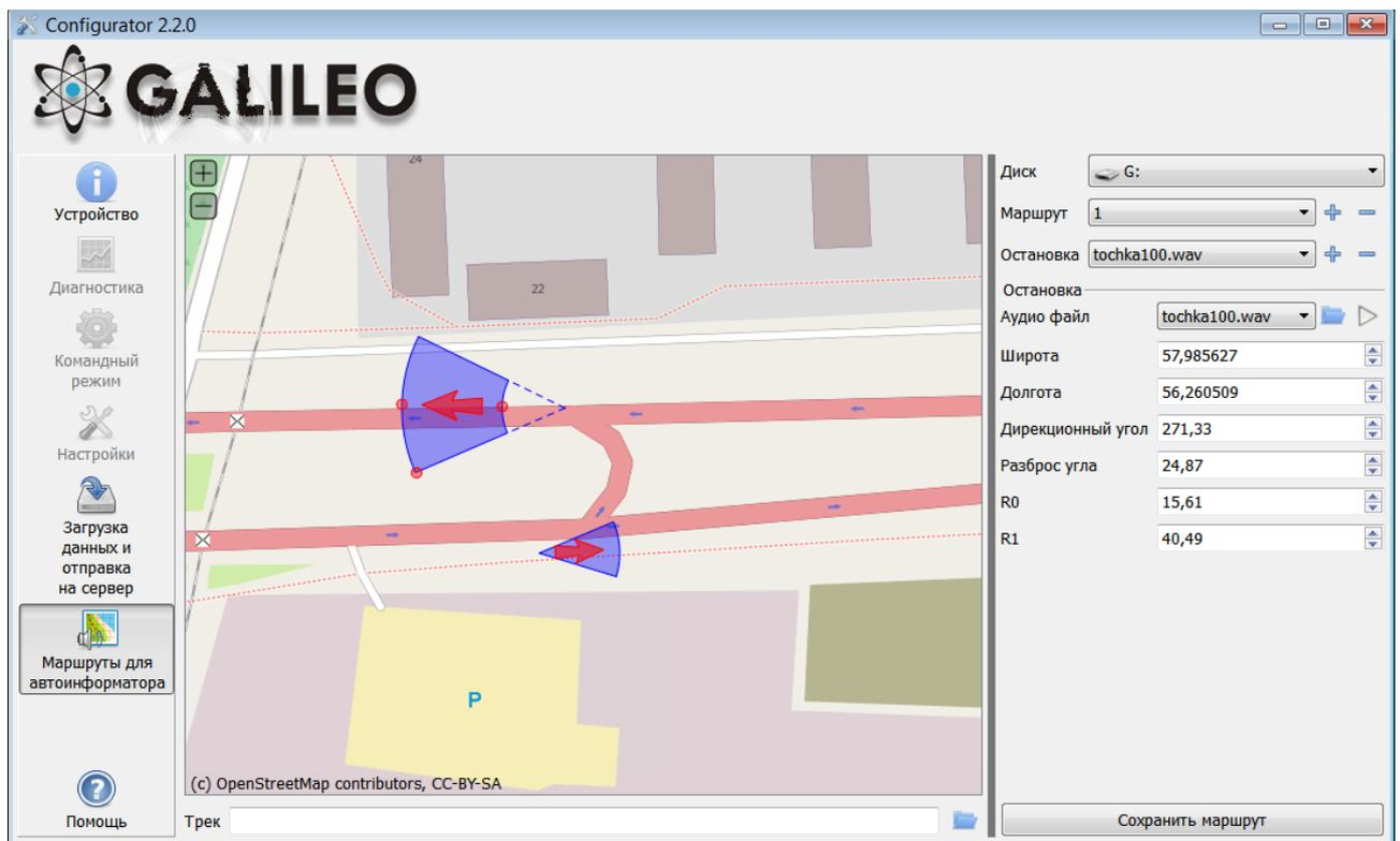
To make sure all zone are correct, download the track developed after a trip. The Configurator supports the tracks uploaded from the internal memory of the Terminal or stored on the micro-SD card in the format csv.
