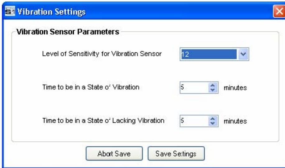
**Level of Sensitivity for Vibration Sensor.** The vibration sensor has a range of sensitivity from 1 to 31 (1 being most sensitive and 31 being least sensitive). The smaller the sensitivity level, the more sensitive the vibration sensor would be to movement.
