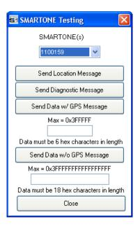
Send Location Message - causes the **SMART**ONE connected to the COM port to obtain a GPS fix and send a Location Message.
