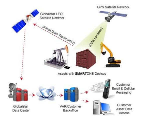
The **SMART**ONE has the unique ability to check its GPS Coordinates at a programmable rate while it is inside of the Change of Location Area without actually sending a message over the Globalstar Simplex Satellite Network.
